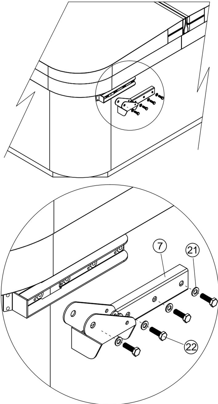
Installation Steps three: install the round tube, and lock with screws
