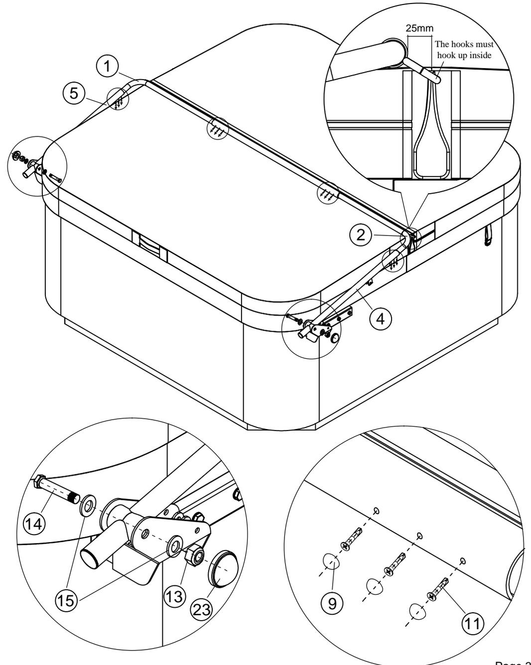
Installation steps four: install the gas rod
