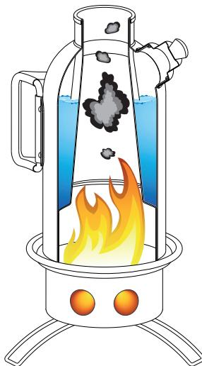
The steam whistle on the cap sounds when the water boils. This is how you have boiling hot water at your disposal with very little effort even on the way and in any weather. Thanks to the three feet, your Petromax Fire Kettle is steady as well as environmentally friendly, leaving no trace from the fire behind.
