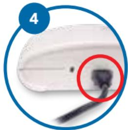
And then plug in the power supply into the CMS™ Gateway Ultra Home Module micro USB power port.
