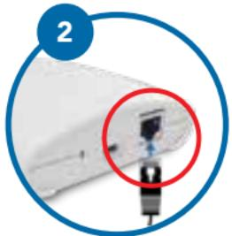
And then plug the other end of the Ethernet cable into the CMS™ Gateway Ultra Home Module.
